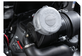
More Muscle - Engine with 35hp and Turbinator Pre-Cleaner
